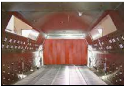
Viewing Windows on Both Sides of the Tunnel
