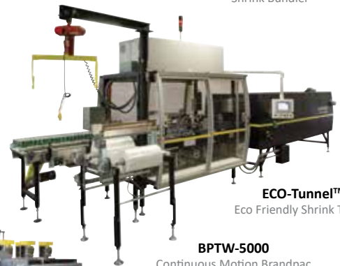
AGR-28 SERIES Intermittent Motion Shrink Bundler Stainless Steel Wash Down
